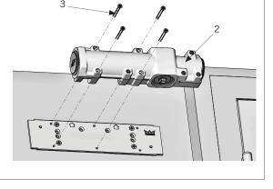
NOTE: Orient pinion (1) closest to hinge.
