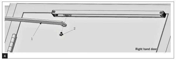
**4.1** Align the arm (1) with the slide shoe of the track channel.
